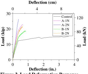
**Figure 2. Load Deformation Response**
